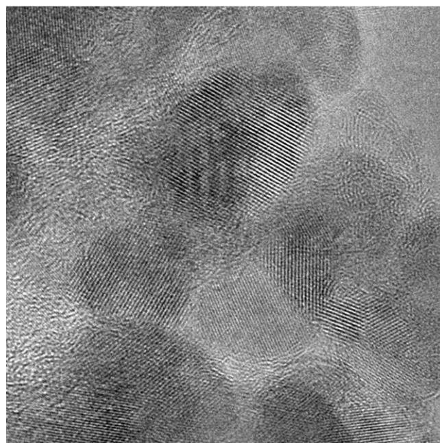
Fig. 19. HRTEM image of \text{FeF}_2 nanocomposite showing 10–20 nm nanocrystallites of \text{FeF}_2 in a matrix of amorphous carbon based on the idealistic metal fluoride nanocomposite schematic shown above.
